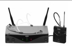
Single channel wireless system with assignable frequency selection. Compatible with the CU400 charging station and AKG's external antenna components. Set consists of SR420 receiver, power supply, PT420 belt-pack transmitter and C555L head worn microphone. Band U1 for Channel 38, band D for licence-free ISM/Channel 70.
