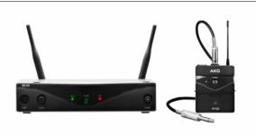
Single channel wireless system with assignable frequency selection. Compatible with the CU400 charging station and AKG's external antenna components. Set consists of SR420 receiver, power supply and PT420 belt pack transmitter with MKGL instrument cable. Band U1 for Channel 38, band D for licence-free ISM/Channel 70.
