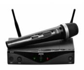
Single channel wireless system with assignable frequency selection. Compatible with the CU400 charging station and AKG's external antenna components. Set consists of SR420 receiver, power supply and HT420 handheld transmitter with D5 capsule. Band U1 for Channel 38, band D for licence-free ISM/Channel 70.
