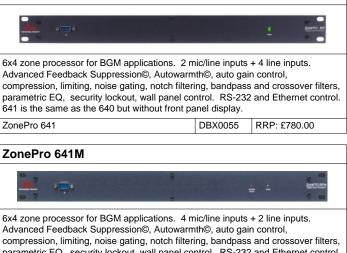
Advanced Feedback Suppression©, Autowarmth©, auto gain control, compression, limiting, noise gating, notch filtering, bandpass and crossover filters, parametric EQ, security lockout, wall panel control. RS-232 and Ethernet control. 641 is the same as the 640 but without front panel display. ZonePro 641m DBX0108 RRP: £875.00
