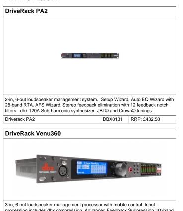
3-In, 6-out loudspeaker management processor with mobile control. Input processing includes dbx compression, Advanced Feedback Suppression, 31-band and 12-band parametric EQ, subharmonic synthesis, delay and noise gate. On the output side, crossover (full range to mono 6-way), 12-band AutoEQ, compression, automatic gain control, tower delays (up to 1s per output) and driver alignment delay. The Venu360 can be controlled by an Android, iOS or Windows mobile device.
