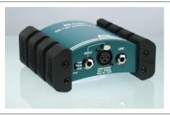
The industry standard DI box. Phantom power and battery supplies as standard. Rugged aluminium extrusion case with robust polyurethane end-cheeks. 1/4" jack and XLR input connections. Input attenuation (-20 & -40dB) making the box suitable for instrument, line or amplifier levels on inputs. Ground-lift switch is provided for a solution to ground-loop problems.
