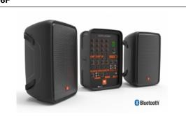
Packaged 8" Two-way PA with powered 8-channel mixer and Bluetooth. Mixer section with four mic/line channels, two stereo line input channels, HiZ input and Bluetooth. On-board reverb. Monitor, subwoofer and headphone outputs. Two two-way speaker cabinets with 8" woofer and 1" neodymium tweeter. Class D amplifier with 300W (2x150W) output. On board DSP limiting. Max output 121dB peak SPL. Frequency range (±3dB) 60Hz - 20kHz. System weights just 17.5kg.
