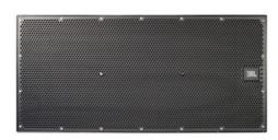
Compact line array optimized for permanent install applications. Advanced technology component transducers for low weight and high output. Outdoor IP55 rated enclosure for protection from dust and water. Comprehensive rigging points for creating a line array configuration. Fiberglass box construction and weatherized components. 2x 2261, 10" diameter LF Drivers & 3x D2415, dual 1.5" diameter annular diaphragm HF Driver. 75Hz - 20kHz frequency response, 100 degrees horizontal coverage.
