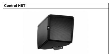
Wide coverage on-wall loudspeaker with Hemispherical Soundfield Technology. One CMMD diaphragm with 1" voice coil, and two splayed CMMD tweeters. 70/100V transformer with taps at 60W, 30W and 15W (plus 7.5W 70V only) and 8-ohm direct. Maximum SPL: 108 dB (peaks of 114 dB). Frequency response ( $\pm 3$  dB) 68 Hz - 18 kHz. Coverage pattern of 180x160 degrees. IP54 rated for indoor/outdoor use. Available in black or white.
