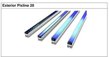
Linear LED video fixture for media facades and creative installations. Can be combined with a wide variety of lenses and diffusers for the right look for every application. Driven by the Martin P3 System Controller family for easy setup and video display, and it is also backwards compatible with DMX for smaller setups. 20 mm pixel pitch. 125 cd per meter calibrated. 80 lumen per foot calibrated. High-quality 16-bit per color image processing technology. Pixel-level brightness
