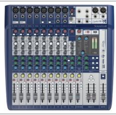
High-performance 12-input small format analogue mixer with onboard effects. 12 channels. 8 Ghost mic preamps, 3-band Sapphyre EQ. 2 dbx limiters on input channels. 3 auxes. 2 mono/1 stereo subgroups. 60mm faders. Single-engine
