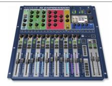
The Si Expression 1 features 16 faders, 16 recallable mic pre amps plus 4 line inputs, 4 internal stereo FX returns, AES in, and a 64x64 expansion slot offering more than enough scope to use every one of the 66 input processing channels. The Si Expression 1 can be rackmounted with the included rack ears.
