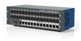
Remote stagebox for Soundcraft Si series consoles. 32 Studer-designed remote controlled mic preamps and AD converters. 12 XLR analogue line level outputs. Dual MADI RJ45/Cat5 connectivity, for 100M runs between stage and mixing console. 3U Rack mount design.
