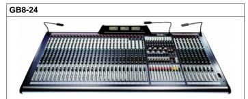
24 mono inputs. GB30 mic preamps with phantom power, phase reverse and HPF filter. 4-band EQ. 4-segment LED meters on every channel. Direct outputs on every channel (pre/post selectable). Four stereo channels. 8 aux sends. 8 sub groups. 4 mute groups. 100mm faders. Dual FOH/monitor modes. 11x4 output matrix. L, R and C outputs. 12-segment LED metering. VU meterpod. Record out with limiter. Internal PSU with external option. Optional 18" gooseneck lights.
