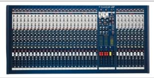
32 channel 4-bus live sound console. GB30 preamps and 4-band EQ with semi-parametric mids. 6 aux sends configrable in pairs as pre- or post-fade for monitor or effects operation. 100mm faders. Comprehensive master section with talkback, two stereo returns and 12-segment group and master LED meters.
