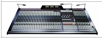
48 mono inputs. GB30 mic preamps with phantom power, phase reverse and HPF filter. 4-band EQ. 4-segment LED meters on every channel. Direct outputs on every channel (pre/post selectable). Four stereo channels. 8 aux sends. 8 sub groups. 4 mute groups. 100mm faders. Dual FOH/monitor modes. 11x4 output matrix. L, R and C outputs. 12-segment LED metering. VU meterpod. Record out with limiter. Internal PSU with external option. Optional 18" gooseneck lights.
