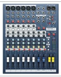
6/2 frame size. 2 configurable auxiliary buses. XLR and jack inputs. GB30 mic preamps and 3-band EQ switch swept mids on mono inputs, 2-band EQ on stereo inputs. TRS insert points on mono inputs and mix outputs. Ten-segment LED output metering. RCA playback inputs and record outputs. Intuitive and comprehensive solo system. Headphone output.
