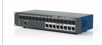
Remote stagebox for Soundcraft Si series consoles. 16 Studer-designed remote controlled mic preamps and AD converters. 8 XLR analogue line level outputs. Single MADI RJ45/Cat5 connectivity, for 100M runs between stage and mixing console. 2U Rack mount design.
