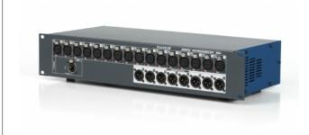
Remote stagebox for Soundcraft Si series consoles. 16 Studer-designed remote controlled mic preamps and AD converters. 8 XLR analogue line level outputs. Single MADI RJ45/Cat5 connectivity, for 100M runs between stage and mixing console. 2U Rack mount design.
