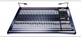
24 mono inputs. GB30 mic preamps with phantom power, phase reverse and HPF filter. 4-band EQ. 4-segment LED meters on every channel. Direct outputs on every channel (pre/post selectable). Two stereo channels. 8 aux sends. 4 sub groups. 4 mute groups. 100mm faders. Dual FOH/monitor modes. 7x4 output matrix. L, R and C outputs. Record out with limiter. Internal PSU with external option.
