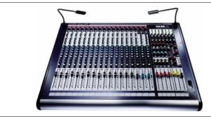
16 mono inputs. GB30 mic preamps with phantom power, phase reverse and HPF filter. 4-band EQ. 4-segment LED meters on every channel. Direct outputs on every channel (pre/post selectable). Two stereo channels. 8 aux sends. 4 sub groups. 4 mute groups. 100mm faders. Dual FOH/monitor modes. 7x4 output matrix. L, R and C outputs. Record out with limiter. Internal PSU with external option.
