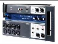
12-input Ui Series mixer. Four XLR combo mic/line inputs, four XLR mic inputs, two channels of Hi-Z instrument inputs, stereo RCA line input. 2 channel USB media player. Two XLR Aux outputs, two 1/4" headphone outputs plus stereo XLR and 1/4" main outputs.
