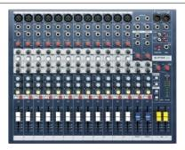
12/2 frame size. 2 configurable auxiliary buses. XLR and jack inputs. GB30 mic preamps and 3-band EQ switch swept mids on mono inputs, 2-band EQ on stereo inputs. TRS insert points on mono inputs and mix outputs. Ten-segment LED output metering. RCA playback inputs and record outputs. Intuitive and comprehensive solo system. Headphone output.
