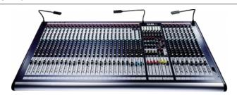
32 mono inputs. GB30 mic preamps with phantom power, phase reverse and HPF filter. 4-band EQ. 4-segment LED meters on every channel. Direct outputs on every channel (pre/post selectable). Two stereo channels. 8 aux sends. 4 sub groups. 4 mute groups. 100mm faders. Dual FOH/monitor modes. 7x4 output matrix. L, R and C outputs. Record out with limiter. Internal PSU with external option.
