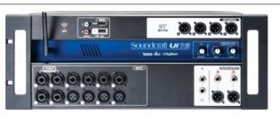
16-input Ui Series mixer. Eight XLR combo mic/line inputs, four XLR mic inputs, two channels of Hi-Z instrument inputs, stereo RCA line input. 2 channel USB media player and 2-channel USB recorder. Four XLR Aux outputs, two 1/4" headphone outputs plus stereo XLR and 1/4" main outputs. HDMI display connection output.
