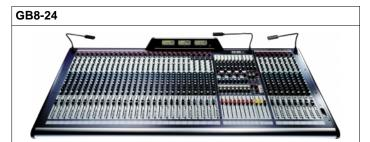
24 mono inputs. GB30 mic preamps with phantom power, phase reverse and HPF filter. 4-band EQ. 4-segment LED meters on every channel. Direct outputs on every channel (pre/post selectable). Four stereo channels. 8 aux sends. 8 sub groups. 4 mute groups. 100mm faders. Dual FOH/monitor modes. 11x4 output matrix. L, R and C outputs. 12-segment LED metering. VU meterpod. Record out with limiter. Internal PSU with external option. Optional 18" gooseneck lights.
